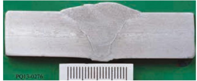
Figure 3. Tie-in weld cross section.
